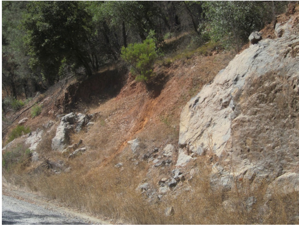
Photograph 1. Typical section of residual soil observed within a road cut southwest of the CRP site
