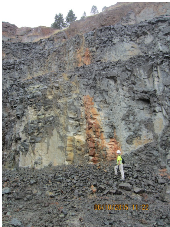
Photograph 9. North facing close-up of quarry shear zone
