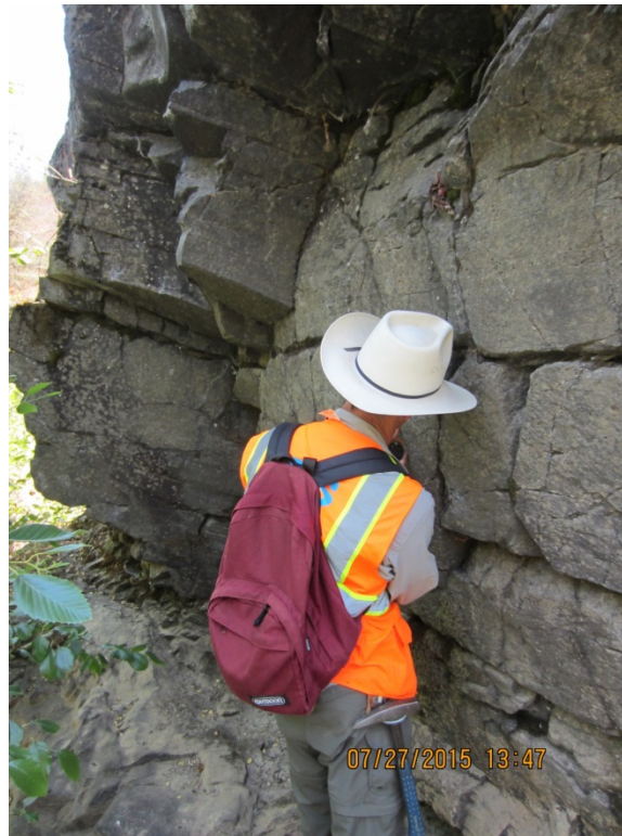
Photograph 5. East facing view of typical discontinuities in outcropping bedrock (massive basalt) at the toe of slope along the south bank of Bear River, near Axis 4
